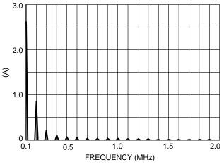
Figure 4. Discontinuous Conduction Mode FFT
