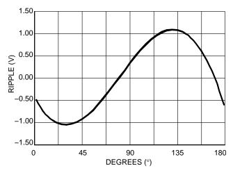
Figure 6. Output Ripple Envelope
