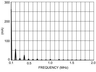
Figure 3. Continuous Conduction Mode FFT
